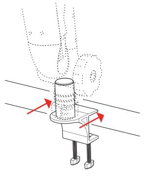
**NOTE:** It is recommended to orient the ShadeFin Mini in the same direction as Clamp Mount. Orienting it away from the mount could cause slippage of the mount.
